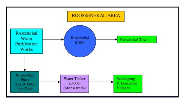
The Schematic Plan below shows the Rossenekal Water Scheme
